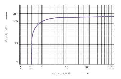
The presented characteristics are valid for dry air at temperatures up to 40  $^{\circ}$ C and an atmospheric pressure of 1013 mbar abs. Tolerance of the characteristics is  $\pm$  10%.
