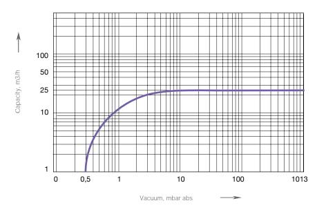
The presented characteristics are valid for dry air at temperatures up to 40  $^{\circ}$ C and an atmospheric pressure of 1013 mbar abs. Tolerance of the characteristics is  $\pm$  10%.
