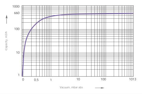
The presented characteristics are valid for dry air at temperatures up to 40  $^{\circ}$ C and an atmospheric pressure of 1013 mbar abs. Tolerance of the characteristics is ± 10%.
